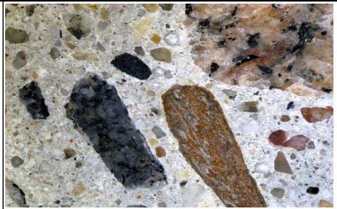
Views at 10x magnification illustrating general views of paste and aggregates. Fields of view about 13 mm.
