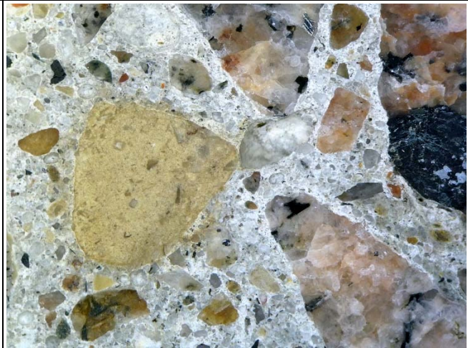
Views at 10x magnification illustrating (left) discoloured paste surrounding a limestone coarse aggregate, with a slight debond observed along its periphery, and an entrapped air void next to the granite aggregates at the upper left; and (right) general condition of paste that encloses granite, gneiss, and limestone aggregates. Fields of view about 13 mm.
