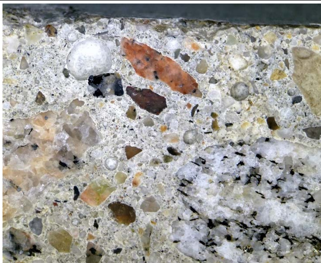
Views at upper/outer face of core, in profile, showing condition of paste. Magn. 10x, fov = 13 mm
