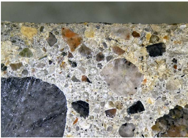
Views at upper/outer face of core, in profile. Slightly discoloured paste at surface. Magn. 10x, fov = 13 mm
