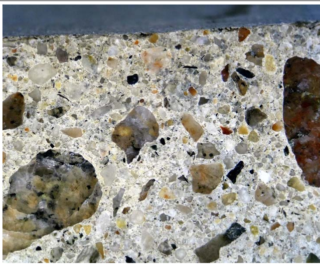
Views at 10x magnification showing profile at outer surface of core (left) and general view of paste and aggregates.. Fields of view about 13 mm.
