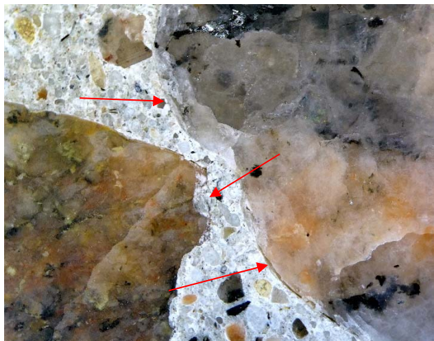
Coarse aggregate particles are partly debonded (arrows) from the paste. 10x mag.
