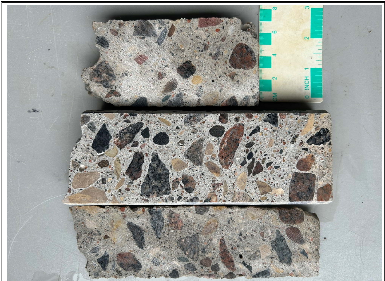
Core after cutting and polishing. Note slightly discoloured paste zone at far right in polished (centre) slab.
