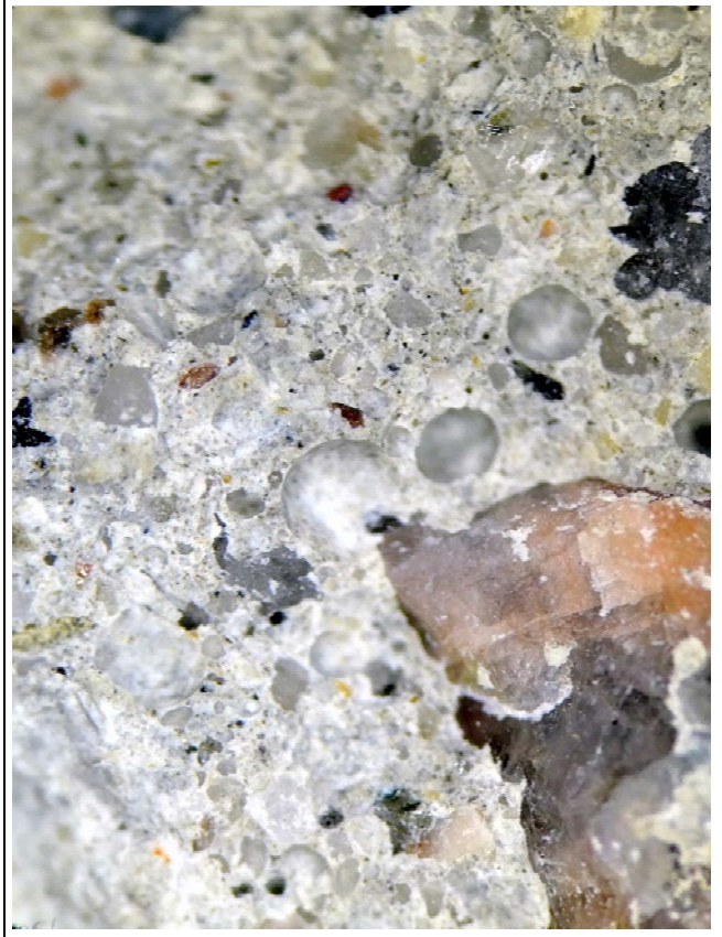
Sandstone coarse aggregate with a vague rim (left image) and view of a rough fractured surface (right image). 10x mag.
