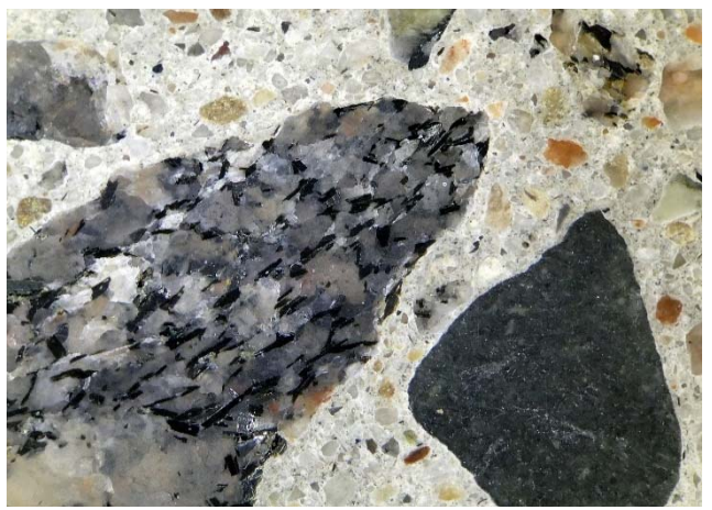
Views at 10x magnification illustrating general views of paste and aggregates. Fields of view about 13 mm.
