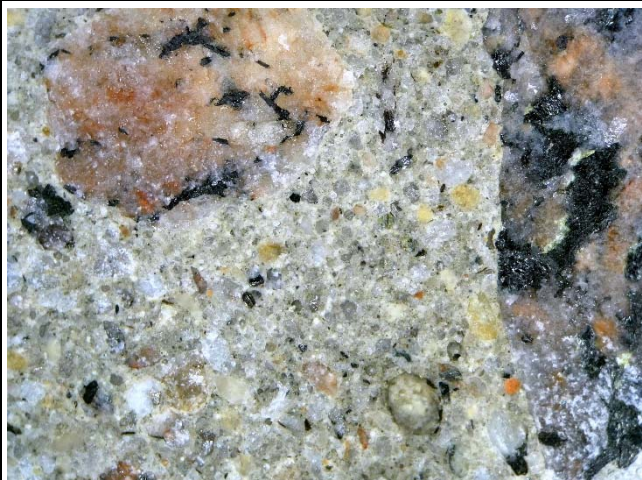
Views at 10x magnification illustrating dense paste containing two granitic aggregate particles, (right) polished surface showing paste that encloses aggregates. Fields of view about 13 mm.
