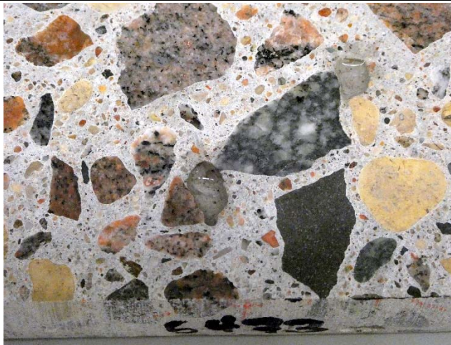
Left: Detail view of the polished core surface, showing granitic, gneissic, quartzite and carbonate coarse aggregates in paste. Right: Profile view at top of core, mag. 10x, field of view about 13 mm.
