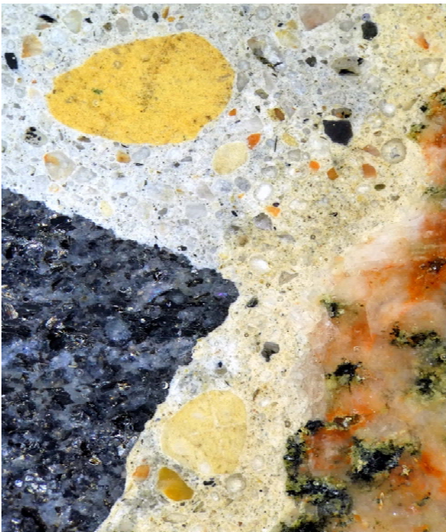
Discoloured, likely carbonated, cement paste at top of sample in left view contrasts with light grey paste seen in the right image, both at 10x magnification. Fields of view about 13 mm.
