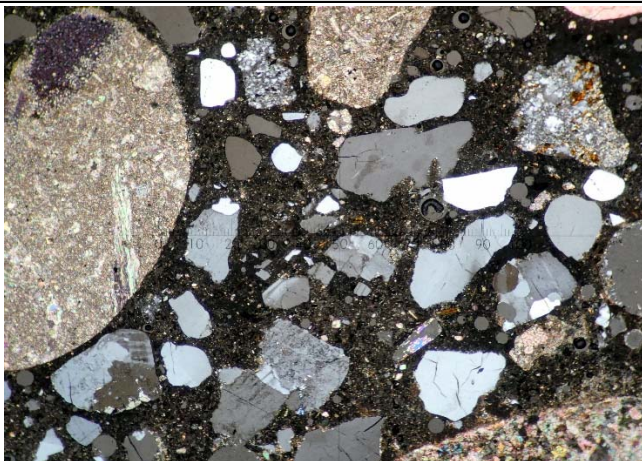
A cross-polarized view showing dense paste; 50 magnification, 3 mm FOV.
