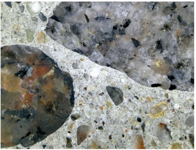
Views at 10x magnification illustrating general condition of paste and aggregates. Field of view is about 13 mm across.
