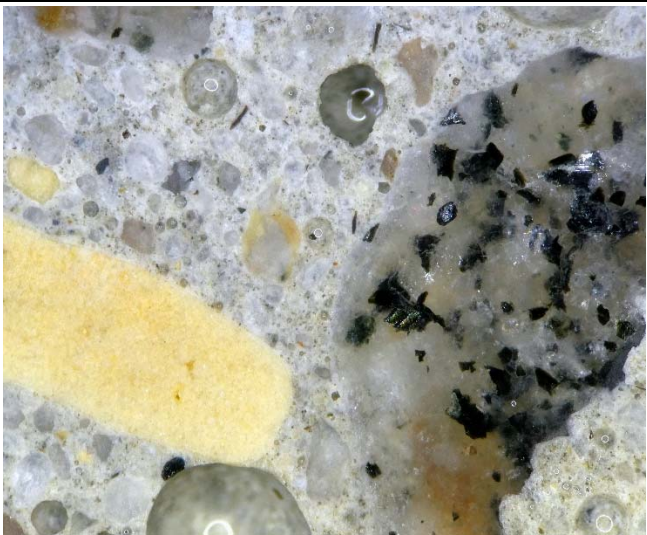
Views at 20x magnification showing dense paste and good encapsulation of aggregates. Fields of view 8 mm across.
