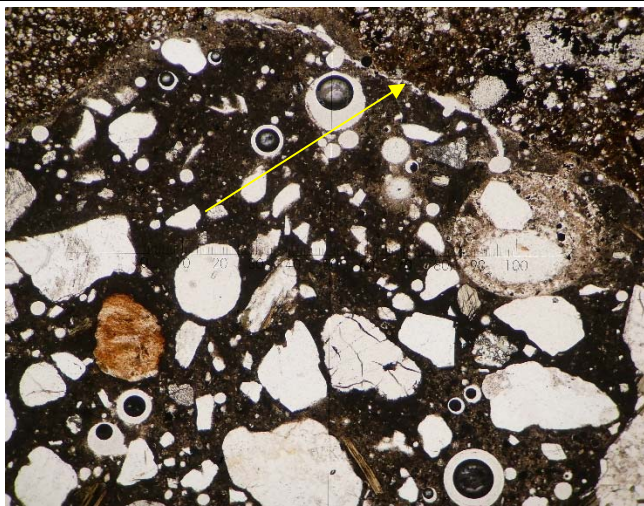
Thin-section images showing fine and very fine microcracks in cement paste; 50x magnification.
