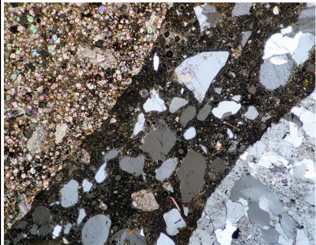
Sound paste is seen between dolomite particle on left and granite on right in this thin-section image; 50x magnification, field of view 3 mm across.
