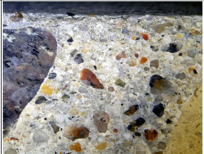
Left: Detail view of the polished core surface, showing granitic, gneissic, quartzite and carbonate coarse aggregates in paste. Right: Profile view at top of core, mag. 10x, field of view about 13 mm.
