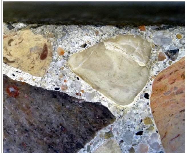
Views at upper/outer face of core, in profile, showing slight attrition paste. Magn. 10x, fov = 13 mm
