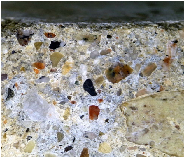
Views at upper/outer face of core, in profile, showing uneven discoloured paste at surface. Magn. 10x, fov = 13 mm
