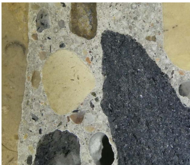
Views at 10x magnification illustrating paste that encloses granite, gneiss, dolomite and limestone aggregates. Fields of view about 13 mm.
