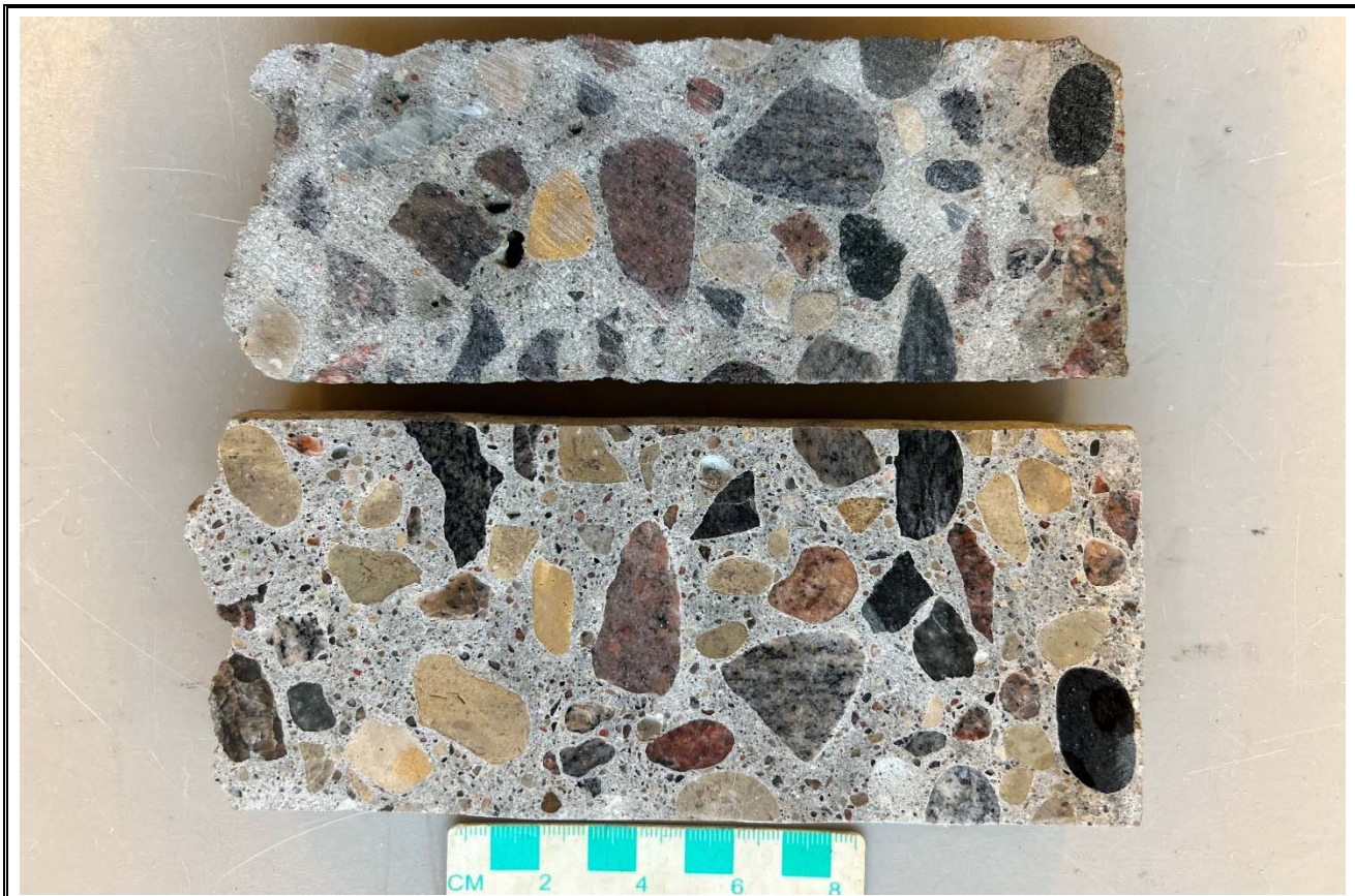
Core after cutting and polishing. Note slight discolouration of paste at outer end.
