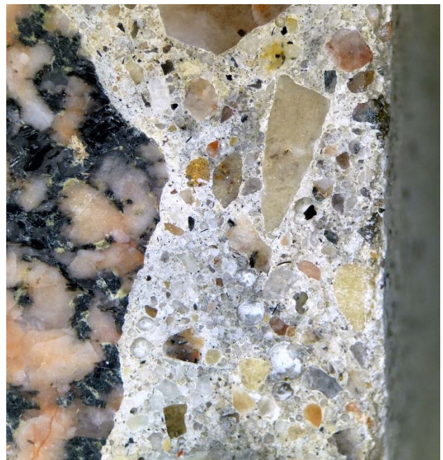
Views at upper/outer face of core, in profile, showing slight attrition of paste on surface and slight discolouration of paste at surface. Magn. 10x, fov = 13 mm
