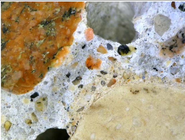
Views at 10x magnification illustrating (left) discoloured paste surrounding a limestone coarse aggregate, with a slight debond observed along its periphery, and an entrapped air void next to the granite aggregates at the upper left; and (right) general condition of paste that encloses granite, gneiss, and limestone aggregates. Fields of view about 13 mm.
