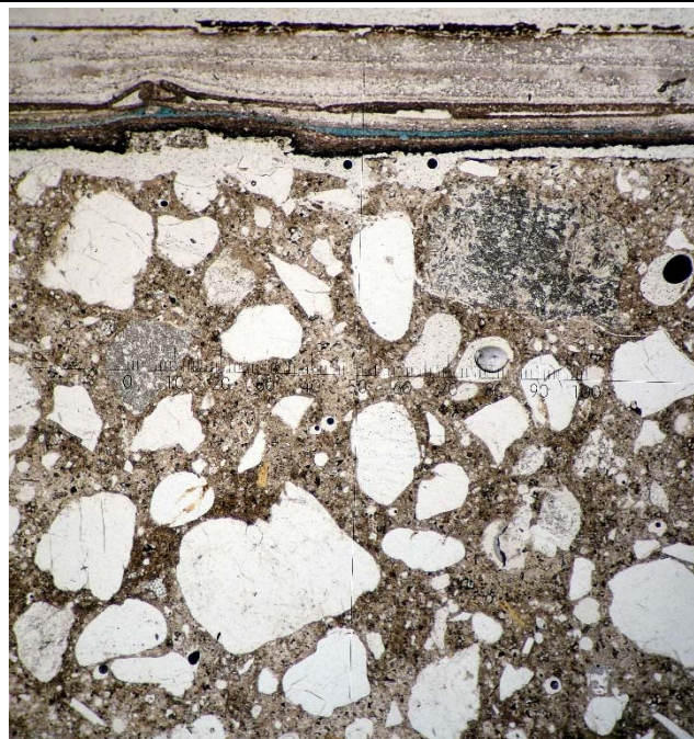
Outer surface of core showing applied layers of paint, etc., at top of image. 50x.
