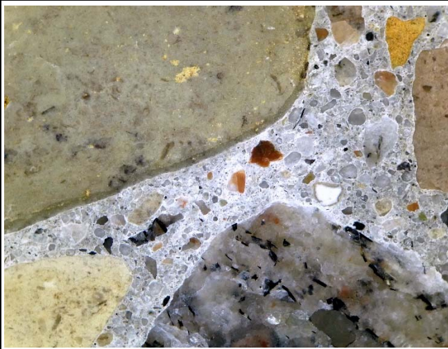
Additional images showing dense paste enclosing sound aggregates; mag. 10x.
