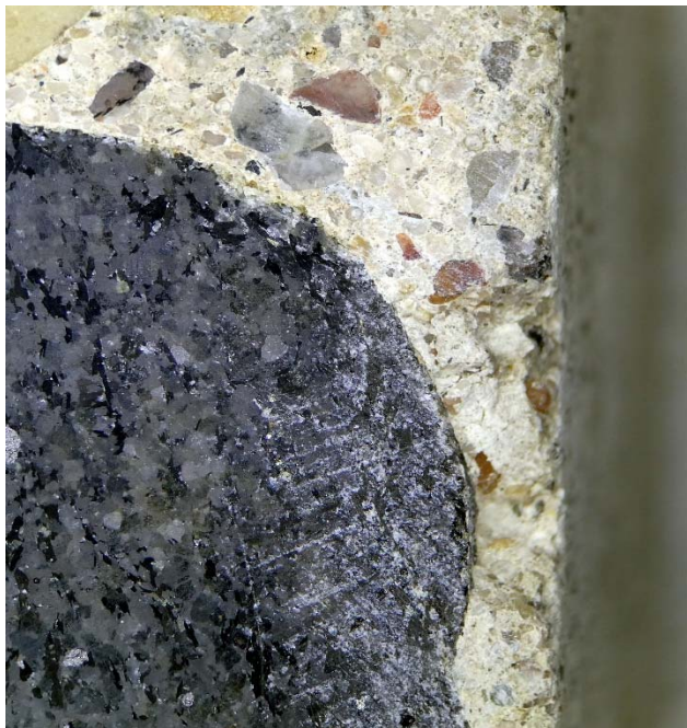
Views at upper/outer face of core, in profile, showing slight attrition of paste on surface and slight discolouration of paste at surface. Magn. 10x, fov = 13 mm
