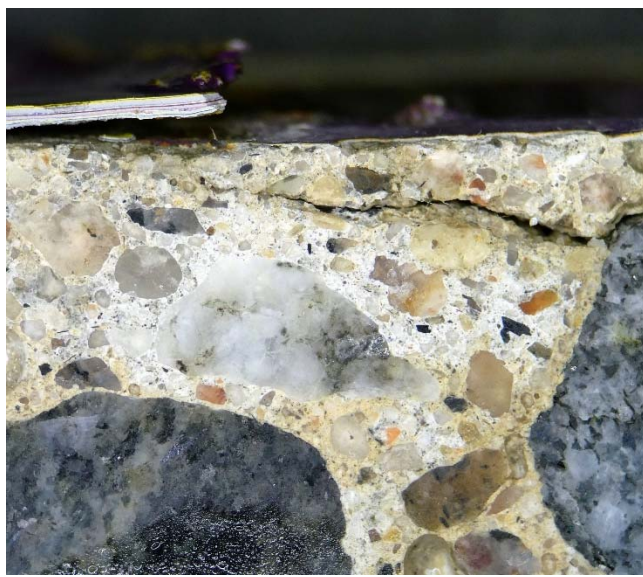
Views at upper/outer face of core, in profile, showing cracks in paste, delamination of paint coatings (left view), and discoloured paste at surface. Magn. 10x, fov = 13 mm
